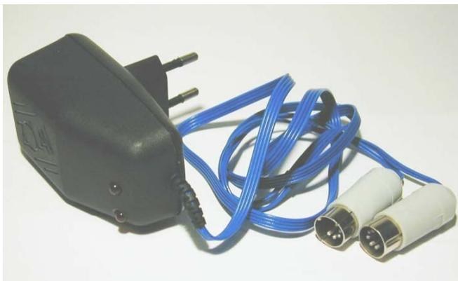
1. The N28 charger is designed for charging all ARDF receivers of COMPACT and SUPERFOX series. One charger can handle any two receivers. The charging current is stabilized at 28 mA. Charging status is indicated by a LED diode.
