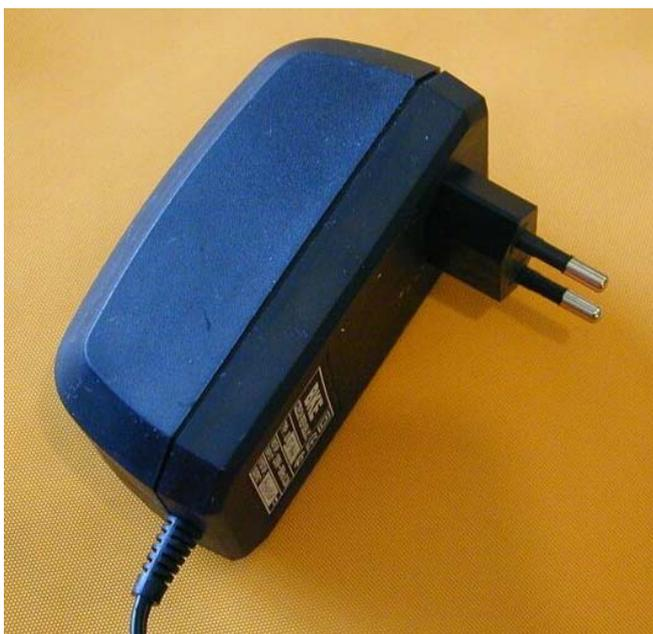
3. The NPB charger is designed for charging one or several transmitters COMPACT 96 or CONTEST 2002. After full charging, it goes to the conservation mode. Charging status is indicated by LED diodes.
