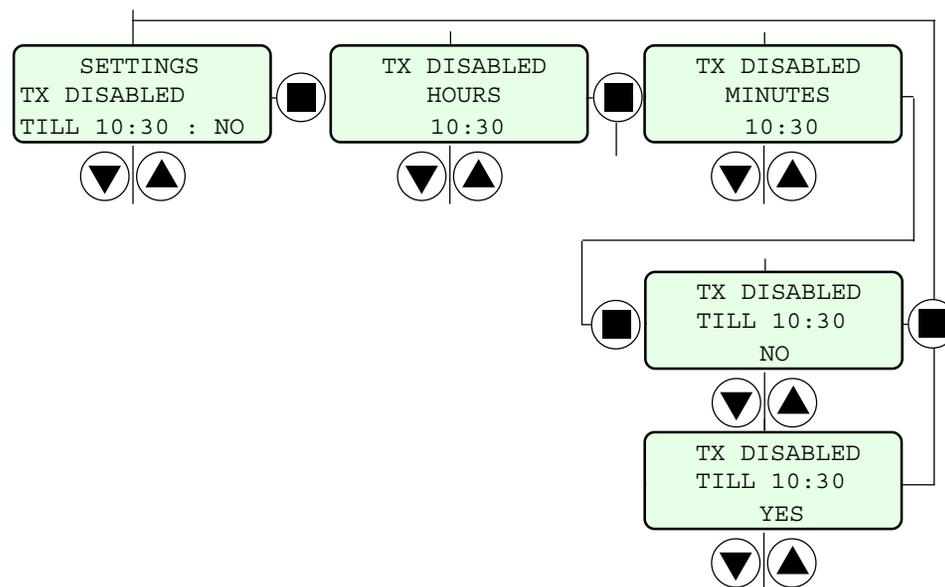
The time at which the transmitter shall commence operation, can be set to any time up to 24 hours in the future.
