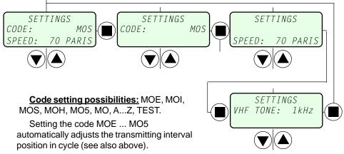
**NOTE: DO NOT USE THE TEST CODE!** The TEST code is intended only for testing and diagnostic purpose. At this setting transmitter generates a continuous carrier, which is allowed only for a short time and into the defined load.
