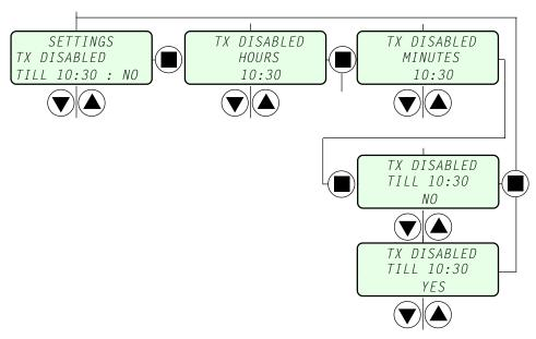
The time at which the transmitter shall commence operation, can be set to any time up to 24 hours in the future.
